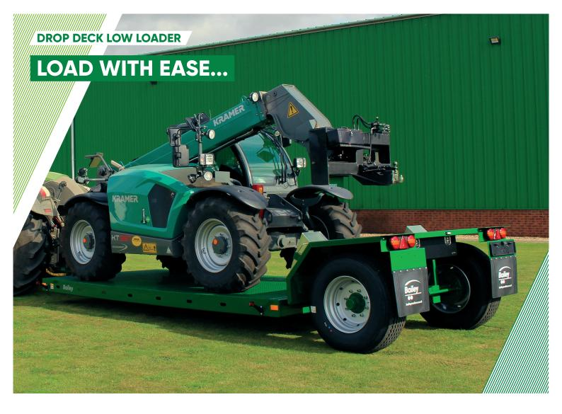
We've designed our range of Drop Deck Low Loader trailers so that the bed of the trailer lowers to the ground to enable easy and quick loading of implements, small crawlers and drills.
