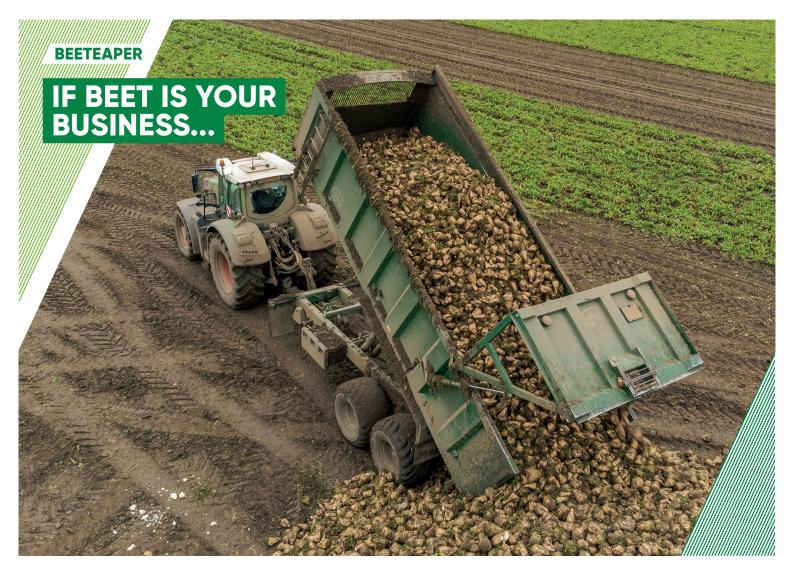
Then you won't beat our Beeteaper trailers. This range is designed especially for transporting and heaping beet and features a unique tipping angle of approximately 60°.
