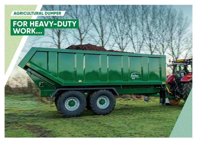
Agricultural Dumpers feature a heavy-duty RHS bottom chassis mounted on a heavy-duty tandem spring unit. This provides additional strength and durability.
