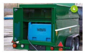
The Adblue tank is located in the rear, lockable compartment **(see 4)**.
