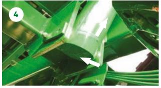
Grease upper and lower tip cylinder pivots.
