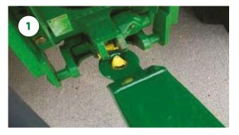
Check the condition of the towing eye for signs of wear or damage.
