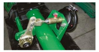
The brakes are applied in a controlled manner, as the pressure builds up behind a rubber diaphragm housed inside the brake chambers **(11)**, and the output forces act on the slack adjusters (or levers) increasing the torque entering the foundation brakes via the camshafts.
