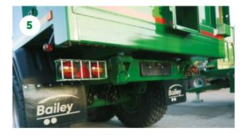
Check lights & reflectors for correct operation & damage.
