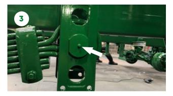
Grease the sprung drawbar pin (where applicable).
