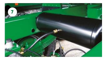
Drain water from air reservoir (where applicable).
