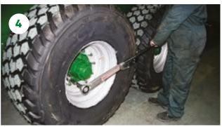
Check wheel nut torque.
