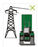
High voltage Do not tip the trailer within 20 meters of overhead high tension electricity cables.
