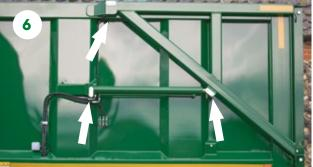
Grease tail gate pivots (3 positions).
