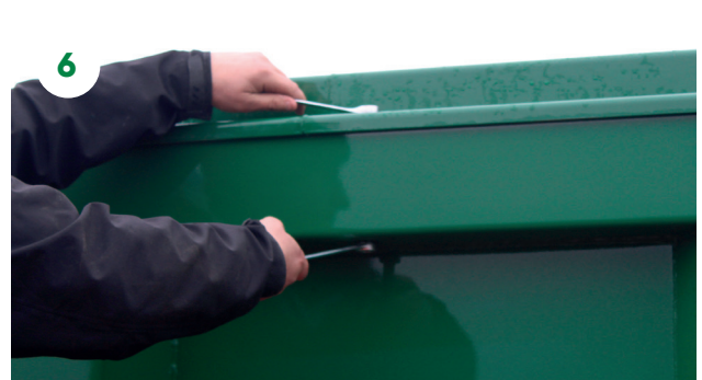
Check side extension bolt security.
