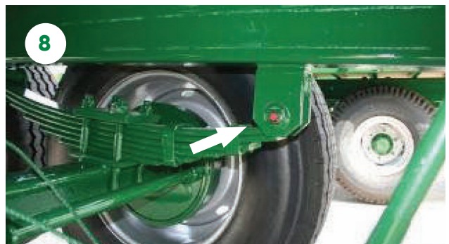
Grease all suspension mounts. Where tandem springs are fitted there are 3 greasers on each side, one on each pin. Where a rocking beam tandem is fitted there are four nipples on the rear of the tandem shaft.
